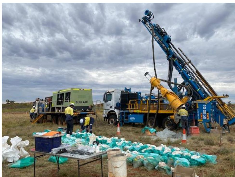
**Figure 2:** RC drill rig at Morto Lago.
